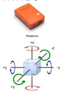
Figure 2. Xsens wireless sensor (top panel) and its 3 dof rotations (bottom panel).
